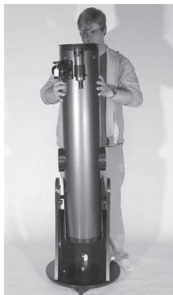
Figure 9. Lift the optical tube and place it into the Dobsonian base so that the altitude bearings rest on the bearing cylinders. Orient the optical tube as shown. Do not bump the encoder connector board or vertical stop when installing the optical tube.
