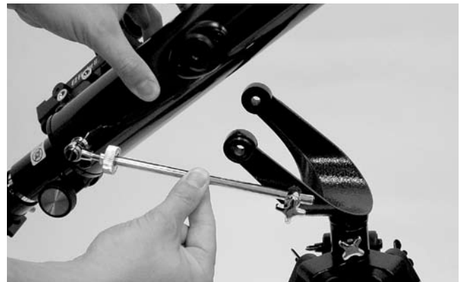
Figure 4. Installing the optical tube in the “yoke” altazimuth mount
