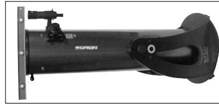
**Figure 8.** Once the base is leveled, point the tube up until the mirror cell comes into contact with the vertical stop. Then, place the carpenter's level across the top of the tube as shown. If the vertical stop is set properly, the top of the tube should also be level.
