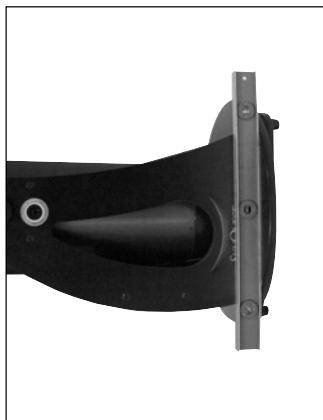
**Figure 7.** Place a carpenter's level on the base as shown. The base should stay level through a 180° rotation in azimuth. Once the vertical stop is set, the base does not need to be level to function properly.
