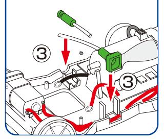
Connect one end of the flexible tubes to the lower nozzle on the storage cylinder and the other end of the flexible tube to the nozzle on fuel cell located nearest to the motor. Connect the other end of the flexible tube on the refueling input valve to the other nozzle located on the fuel cell. Connect the purging valve tube to the upper nozzle located on the storage cylinder. Make sure all tubes are properly positioned as in diagram.
